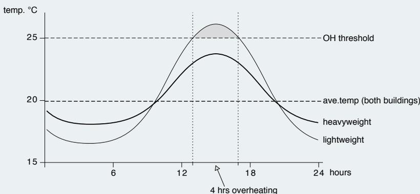
Dense materials have more effect than lightweight materials in providing thermal mass, but it is essential that the mass is accessible from the occupied space and/or the space in which the gains are made (Figure 2).
