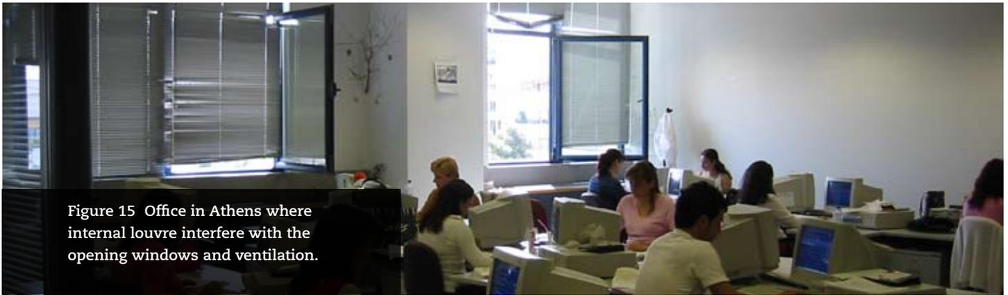
Figure 15 Office in Athens where internal louvre interfere with the opening windows and ventilation.
