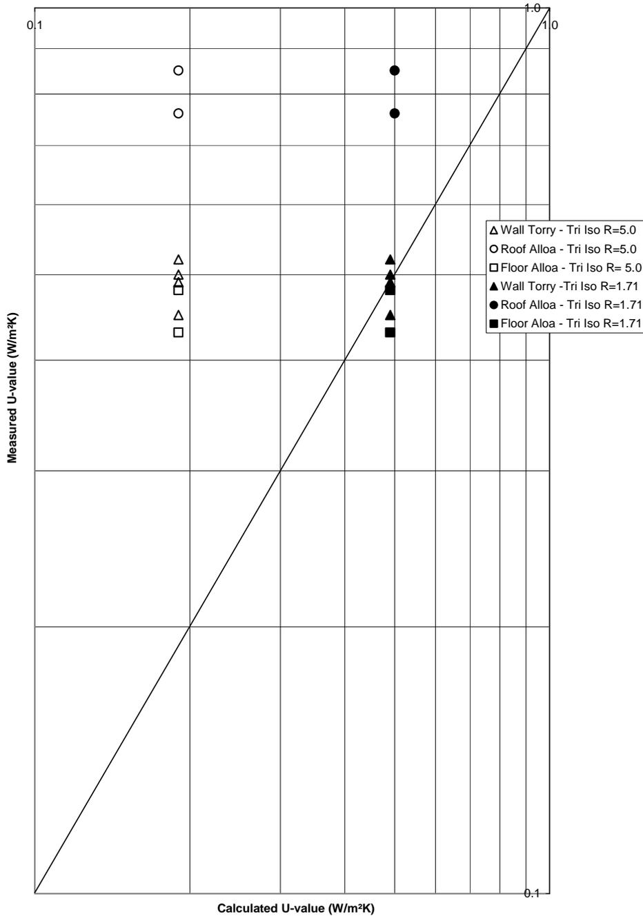
Figure 2: Comparison of measured and calculated U-values
